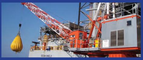
ALATAS supply water bags and load cells for both dynamic and static load tests for Marine Offshore & landbased cranes. ALATAS crane load tests are **ALATAS** performed as per designed protocols, matching individual crane models set out by the manufactures. A certificate is issued upon successful completion.
